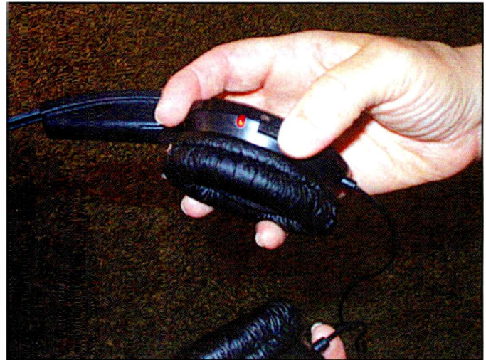
The NoiseBuster headphones' on/off switch is located on the edge of one earpiece.
