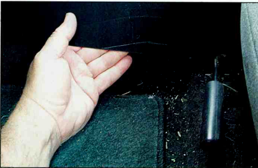
The RAM or w9iix.com mounts can be bolted to the plastic transmission hump mount in this vehicle. It takes a cool day and some patience to drill the holes and reach up under the plastic with the nuts and lock washers.
