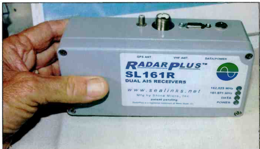
The two-channel AIS receiver for shipboard collision avoidance.
