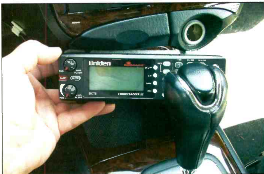
The Uniden BCT-8 with regular duty-type Velcro mounted at a good viewing angle in the Sonata.
