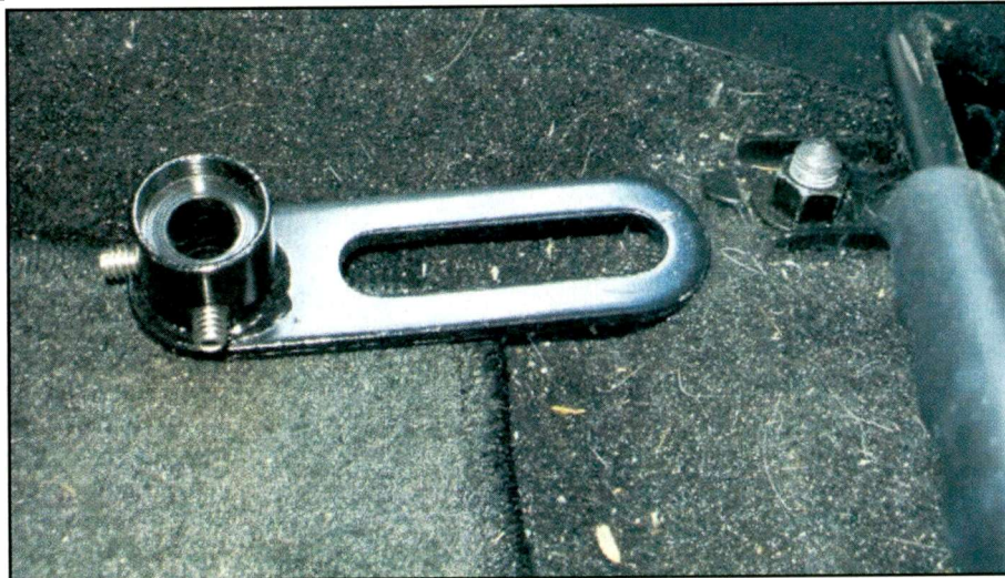
While I was unable to satisfactorily bolt the RAM pedestal bracket plate to the car's seat bolt, you might have better luck in your vehicle. A long flexible, yet sturdy, arm extends upward from this base to which you attach an optional RAM plate that conforms to most radios.
